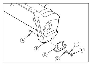
Figure 13. Skid Shoe Installation
